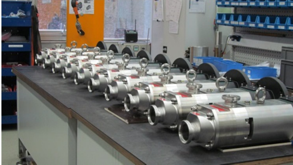
Final assembly of HYGHSPIN 50 pumps for a US customer
